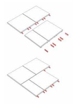
The Terrasoft system plugs are an installation facilitator with dowel character and serve for optimum position assurance.
